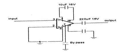
Fig 3.2- A simple LM386 amplifier
