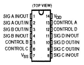
Fig 3.9- Pin assignment of 4066B
