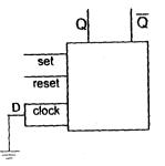
Fig 3.6- Conversion of the D-latch to SR-latch
