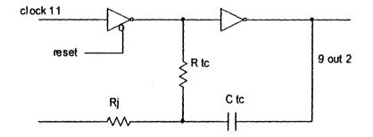
Fig 3.4- Oscillator circuit using RC configuration
