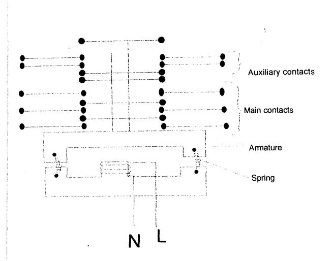
Fig 3.1 Electromagnetic contactor
