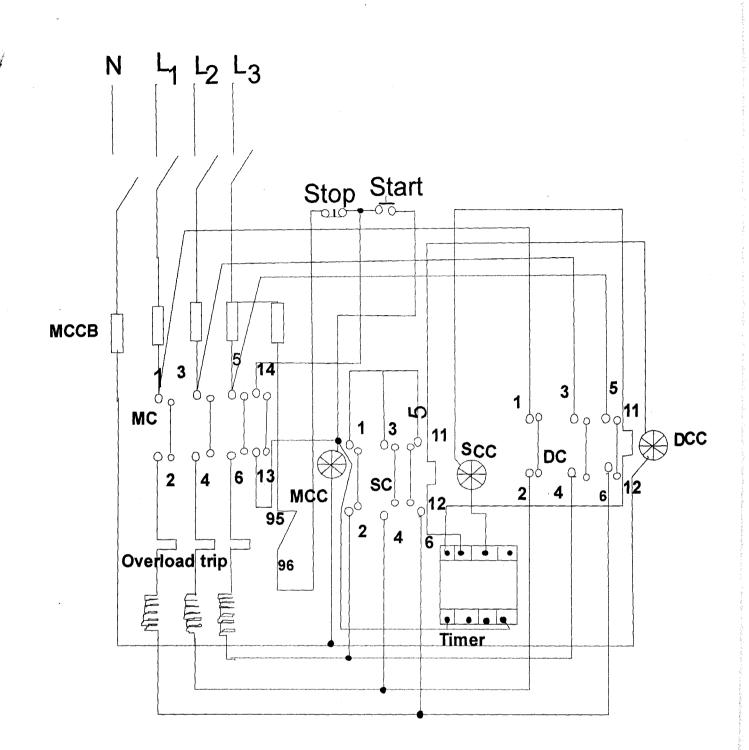
Fig.3.4 Connection diagram of An Automatic Star-Delta Starter.
