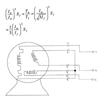
Fig2.1 3-phase motor connected for wye start.
