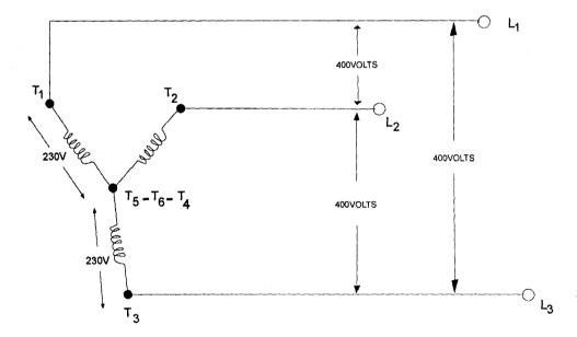
Fig2.1 a star arrangement in which each of the phase windings receives approximately 58% of the supply voltage
