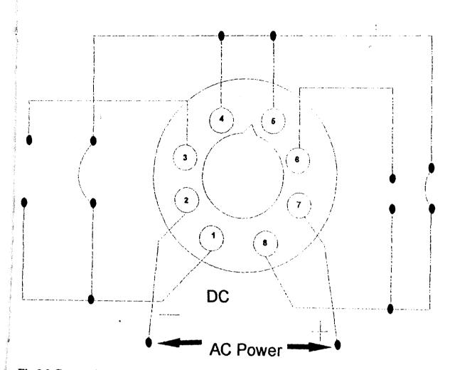
Fig 3.3 Connection diagram of the timer
