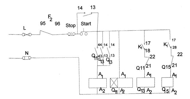
Fig.1.2 Automatic Start-Delta Starter Control circuit.
