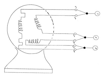
Fig 2.2 a  $3\Phi$  motor connected for delta run.
