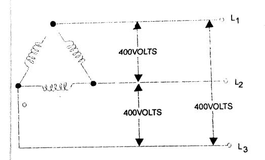
Fig 2.3 a delta ( $\Delta$ ) mesh arrangement with each phase winding receives exactly the applied voltage.
