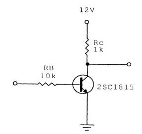
Fig. 2.6 Transistor Amplifier
