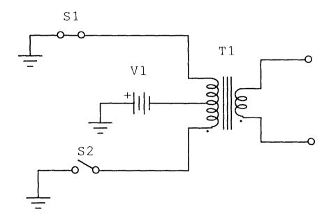
Fig 1.1 Square wave inverter, state 1.
