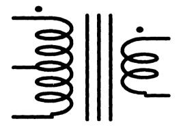
Fig.2.3 Step-up transformer
