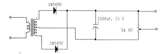
Fig. 2.5 Charging circuit.
