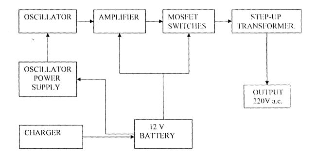
Fig. 2.1 Block Diagram of the project.
