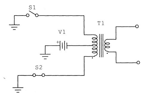
Fig 1.2 Square wave inverter, state 2.
