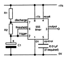
FIG 3.3 555 astable circuit
