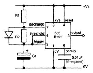
FIG 3.4 555 astable circuit with diode across R2
