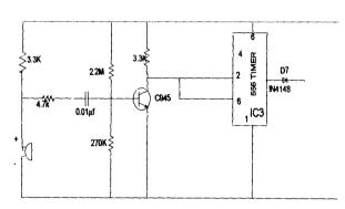
Fig 3.8 Sound Detector System
