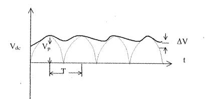
Fig.3.3.2.a filtered voltage wave form.
