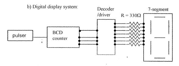
Fig 3.9.2.c.block diagram of a simple digital display system.
