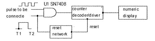
Fig 3.8.a Block diagram of AND gate (7408) used for gating 7490.
