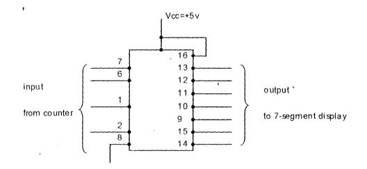
Fig.3.8.c Circuit diagram of the 7448 decoder/driver.
