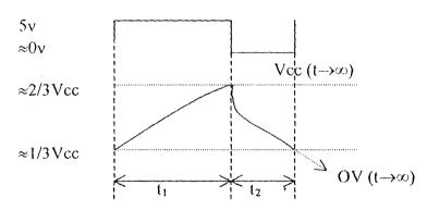
Fig. 3.7.c wave form analysis for one cycle.
