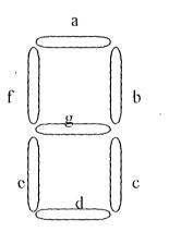
Fig 3.9.2.a Seven segment LED display (FND 360).
