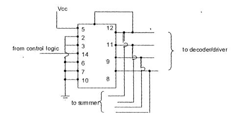
Fig 3.8.b Circuit diagram for 7490 counter.
