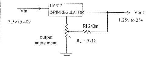
Fig 3.4.a .Variable voltage regulator (LM317).
