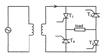
Fig. 2.12a Showing a Bridge Full wave Connection.
