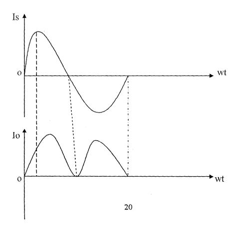
Fig. 2.12d showing the output wave forms of a full wave rectifier.
