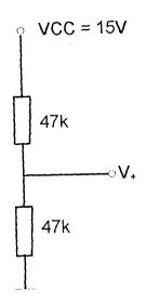
Fig. 3.4 showing the biasing arrangement of the pre-amplifier stage.
