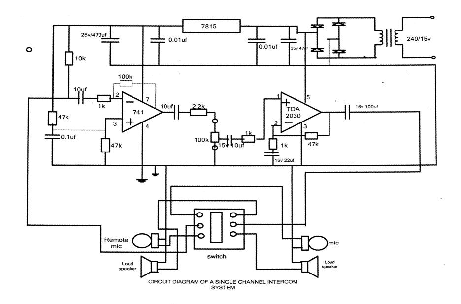
The basic function of the coupling capacitors is to remove any d.c. components in the signal from affecting the d.c biasing of the operational amplifiers. Also, in figure 3.7, the capacitor 16V 10µf is a coupling capacitor which coupled the regulated output of the potentiometer into the power amplifier (TDA2030). Capacitor 16V 10µf serves as an earthing capacitor.
