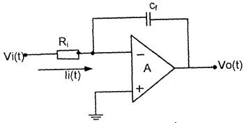
Fig. 2.8 showing op-amp as an integrator.
