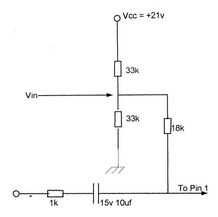
Fig. 3.8 showing the biasing arrangement.
