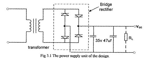
From the module above which represents the power supply unit, the following calculation can be deduced;
