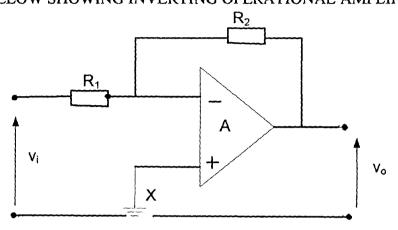
Fig. 2.3 Inverting operational amplifier.
