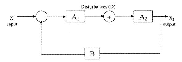
Fig. 2.11 showing the unwanted effect in amplifier.
