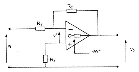
Fig. 2.5 Input and output impedance of an inverting amplifier.
