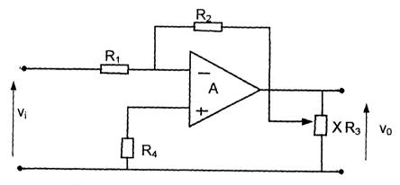
Fig. 2.4 showing the gain of the inverting amplifier.
