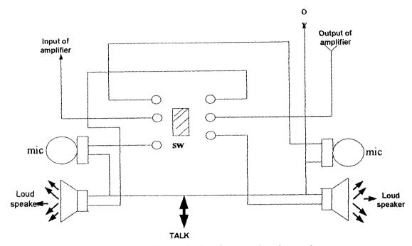
Fig. 3.10 showing the loudspeaker and microphone unit.
