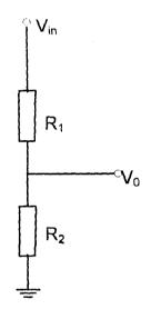
Fig 3.5 showing biasing arrangement.
