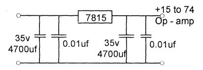
Fig. 3.2 Showing regulation unit connections.
