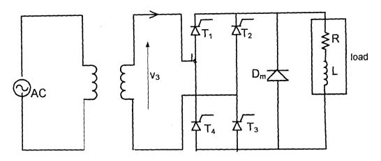
Fig 2.13a Shows a Bridge Converter Circuit.
