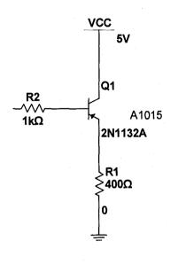
Fig. 3.3 Design of relay driver
