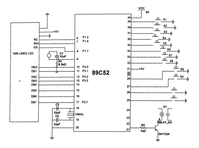
Fig 3.4 Circuit diagram showing the design and construction of an electronic timed mosquito fleeting
