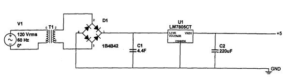
fig. 3.2 circuit diagram of power supply unit
