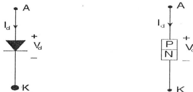
Fig 2.7: Schematic Diagram Of A Diode
