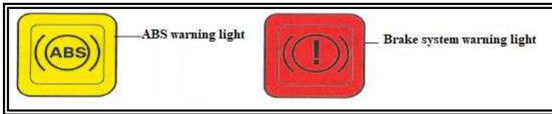
Figure 2.5: ABS and Brake system warning lights.
