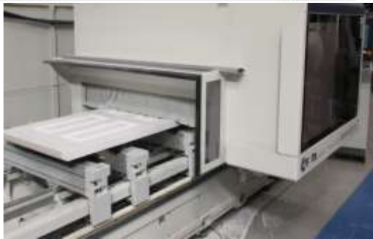
Figure 2.4 CNC machine for doors CNC machine
