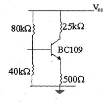
Fig 3f Final common base circuit.
