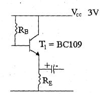
Fig 3c: The common collector stage
