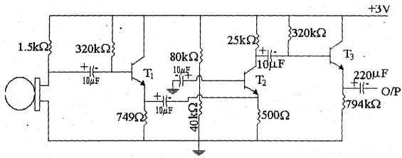
Fig 3g: The final circuit of module 1
