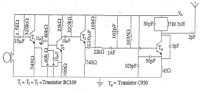
Fig. 3m: The final FM transmitter circuit
