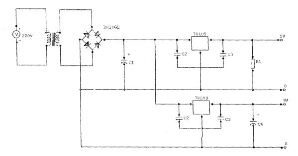
Fig 3.5 full diagrams of the power supply.
