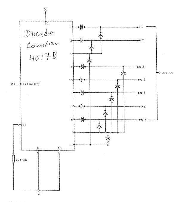
Fig 3.9 Control unit (A) circuit diagram
