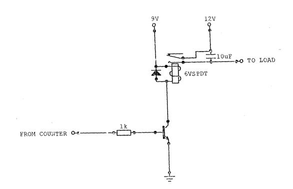
Fig 3.10 switching circuit diagram
