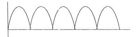
fig 2.7 (a) full – wave rectifier output wave form The output wave form of the filter is shown below
