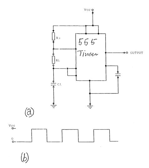
Fig 2.3(a) Astable 555 timer (b) output waveform of an astable 555 timer.
