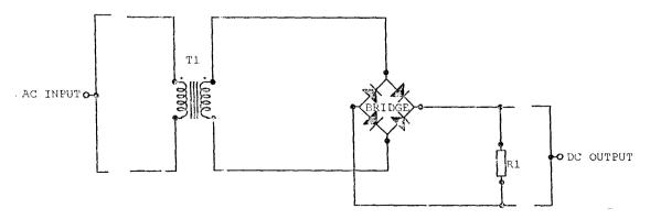
Fig. 2.6 full wave rectifier with resistive loade
