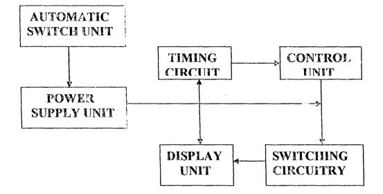
Fig 3.1 Block diagram of automatic electronic display board.
