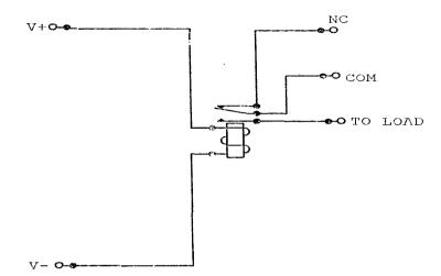
Fig 2.5 Typical structure of a relay
