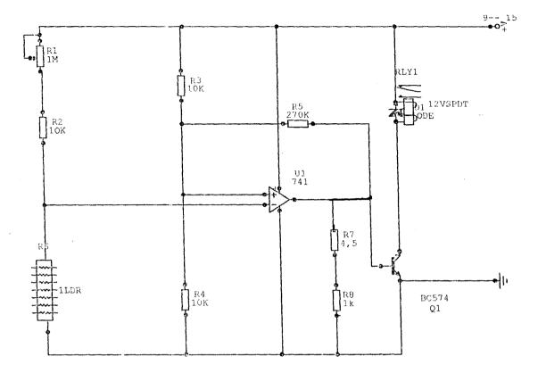
Fig 3.2 Automatic switch circuit diagram
