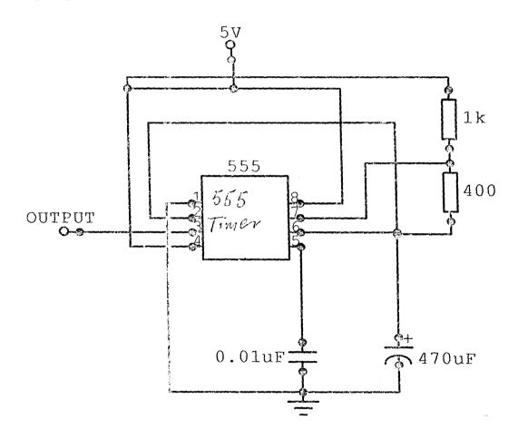
Fig. 3.8 Timing circuit (B) diagram
