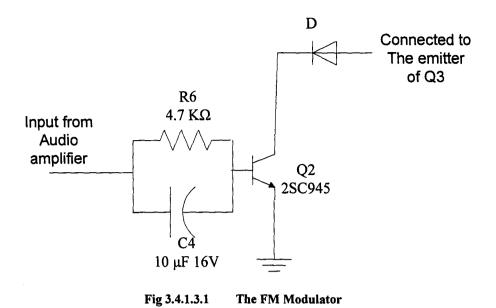
An NPN transistor (2SC945 same that used in the audio amplifier) is connected in a common emitter mode. The base of the transistor Q1 is coupled to the audio amplifier by an impedance circuit of  $4.7k\Omega$  and 16V,  $10 \times 10^{-6}$  Farads connected in parallel, while the collector is connected to emitter of the oscillator's transistor through a diode D.
