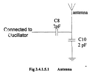
A copper wire was attached to the oscillator through a coupling 2pF capacitor C9. Another capacitorC10 of value 2pF was used to ground the wire; the capacitor C10 was used as filter capacitor. The length of the antonna was not calculated.
