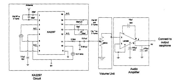
Fig 3.4.2.1 (b) Receiver circuit diagram
