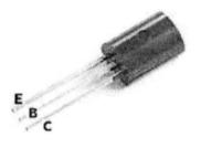
Plate V: A transistor
