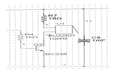
Fig. 9: The driver transistor in the circuit
