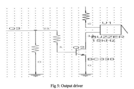
For an NPN transistor, the collector – emitter terminals allow conduction if sufficient base current is driven through the base to saturate it. However, a value of 9V was used in this circuit. At this voltage, the current through the buzzer is determined as illustrated below:
