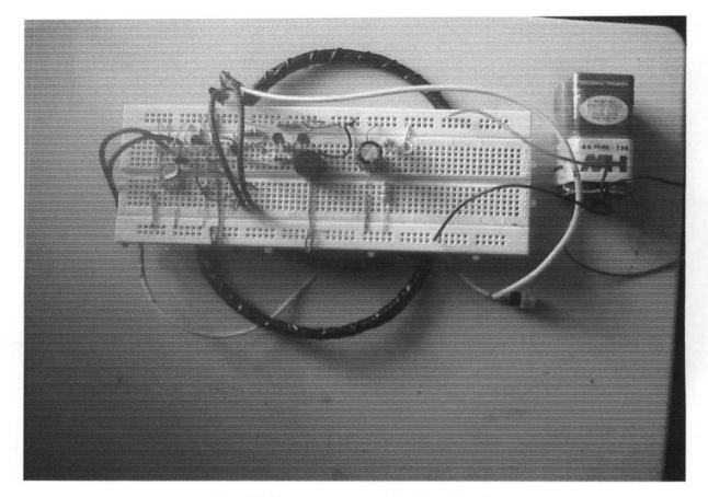
Plate VI: Temporary construction (breadboard)
