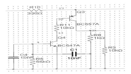
Fig. 8: voltage controlled oscillator of the circuit
