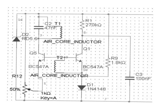
Fig. 7: Feedback oscillator of the circuit
