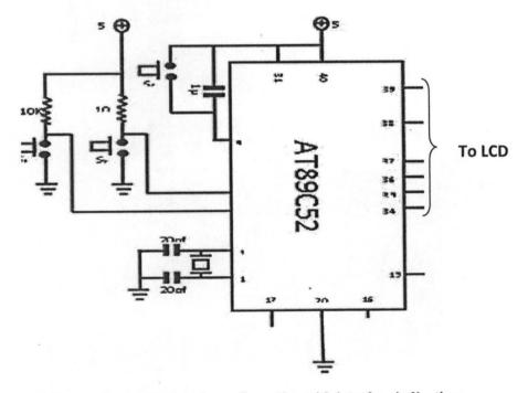
Figure 3.4: basic microcontroller pin configuration with interface indications
