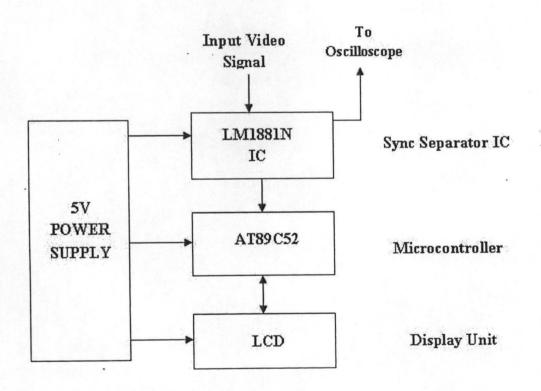
Figure 3.1: Block diagram of the Video Line Selector
