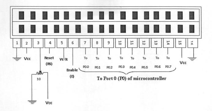
Figure 3.3: LCD pin configuration with microcontroller interface indications
