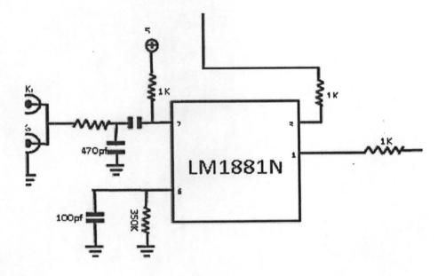
Figure 3.2: The circuit diagram of the Synchronization Separator Module
