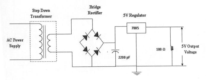
Figure 3.5: Power Supply Unit
