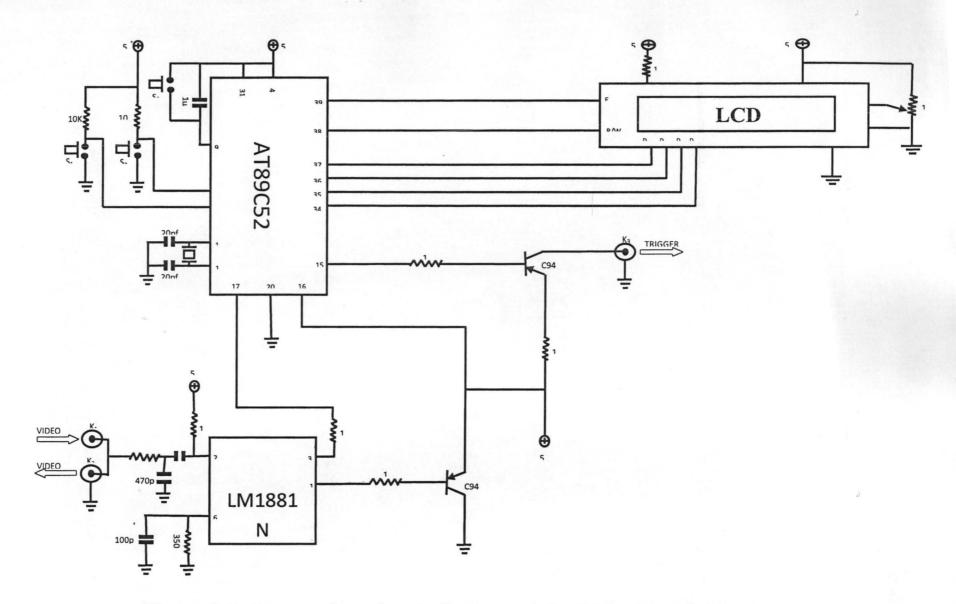
Figure 3.6: the complete circuit diagram of the Video Line Selector
