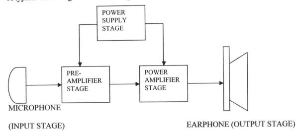
Fig. 3.1 Block diagram of a hearing aid.
