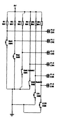
Figure 3.14: schematic diagram of keypad unit
