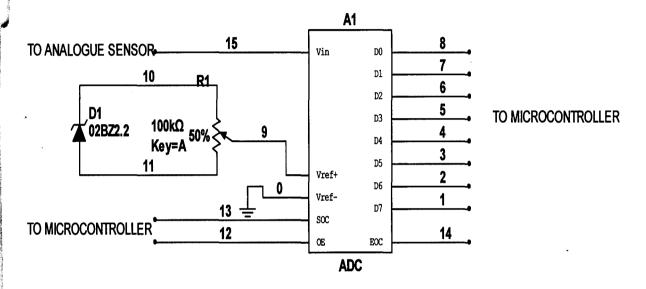
Fig.3.8: schematic circuit diagram of ADC unit
