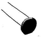
Figure:2.3 cadmium sulfide (CdS) stereogram
