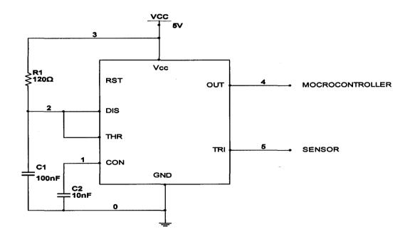
Fig.3.6: Schematic of a 555 timer in monostable
