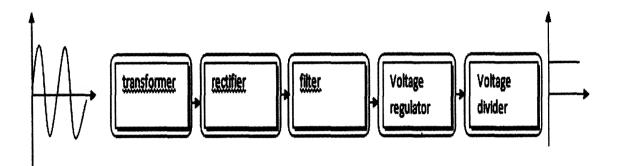
Figure:2.4 Block diagram of power unit
