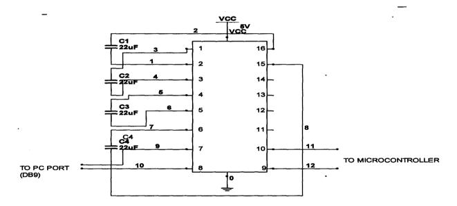
Figure 3.10: schematic diagram of transceiver unit
