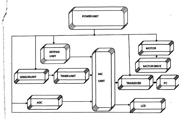
Fig 3.1: Solar tracker block diagram
