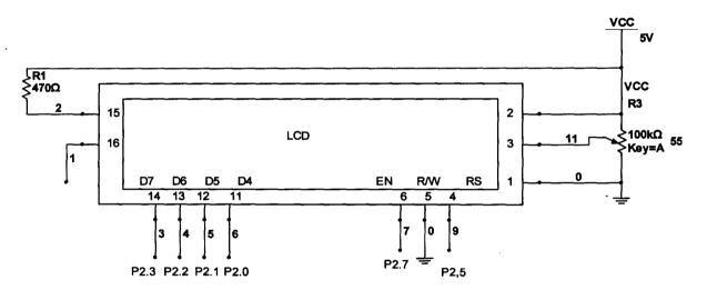
Figure 3.12: schematic diagram of display unit
