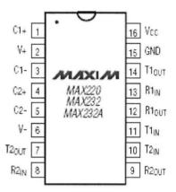
Fig3.3: Pin diagram of MAX232
