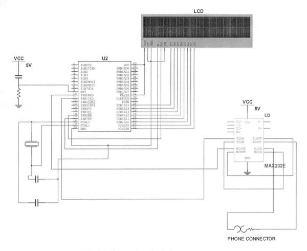
Fig. 3.6. The complete circuit diagram
