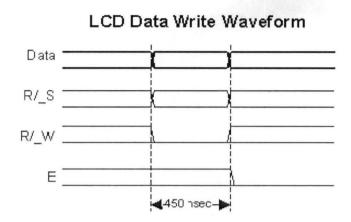
Fig. 3.7 LCD data write waveform.
