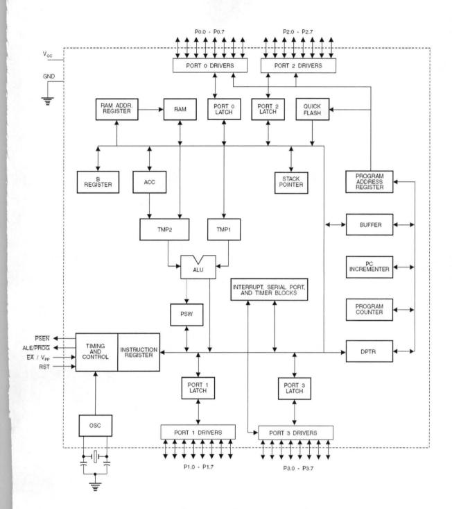
Fig3.2: Internal Architecture of AT89C52
