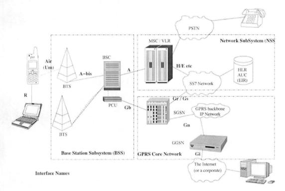
Fig 2.1 Network structure of a GSM system
