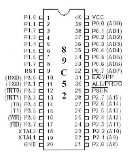
Fig 3.1 Pin Diagram of 89C52
