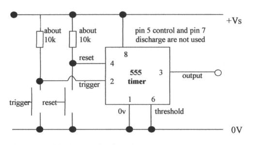
Fig 2.7 Bistable circuit mode of 555 timer
