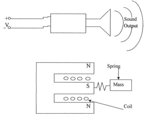
Fig 2.4 Loudspeaker and its longitudinal section
