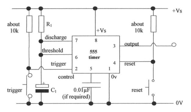
Fig 2.6 A Monostable mode of a 555 timer
