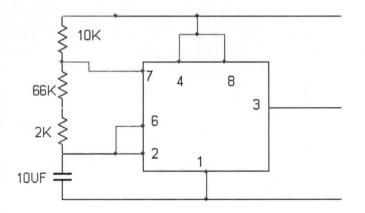
Fig 3.4a Oscillator circuit for the first 555 timer
