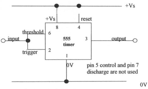
Fig 2.8 The Buffer circuit of 555 timer
