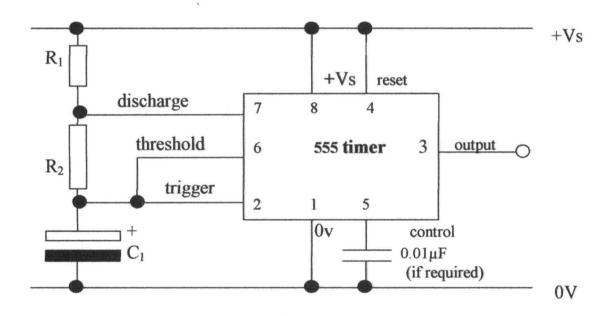
Fig 2.5 An Astable circuit mode of a 555 timer
