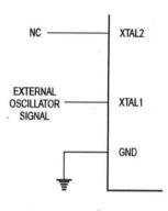
Figure 2.3. external clock drive configuration
