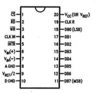
Fig. 1.0 Diagram of ADC0804 showing pin configuration
