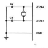
**Figure 2.2.oscilator connection**
