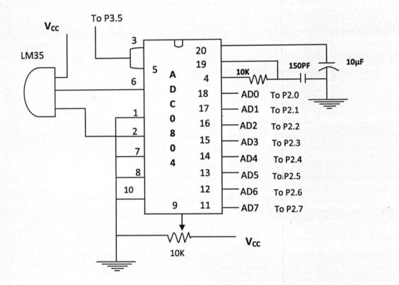
Fig. 3.2 Diagram of the temperature unit
