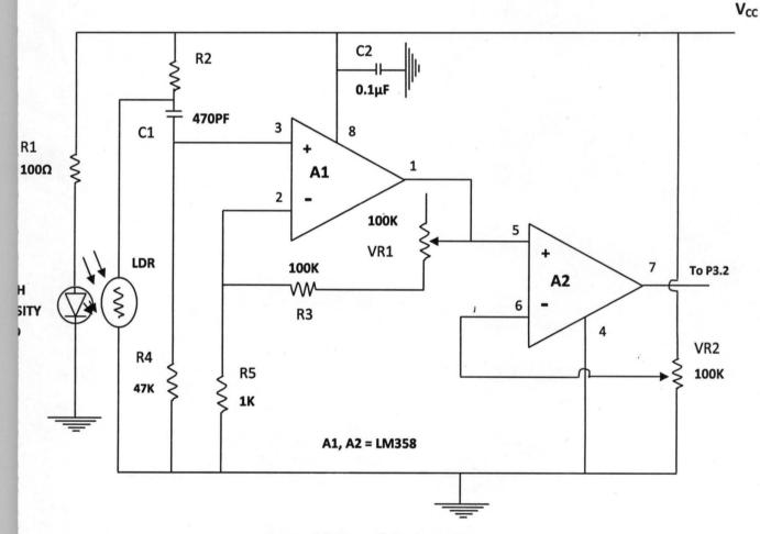
Figure 3.3 Heart Rate circuit diagram
