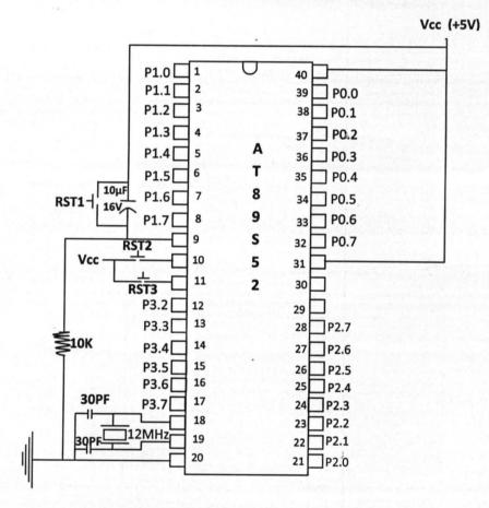
Figure 3.5 basic microcontroller pin configuration with interface indications
