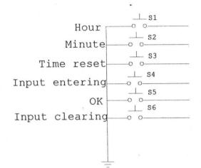
Fig3.3 Circuit Diagram of User's Input Keys
