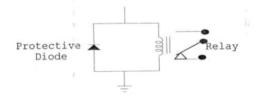
Fig 3.7 Illustration of Protective Circuit
