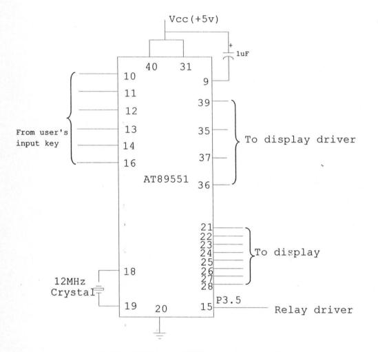
Fig 3.4 Circuit Diagram of Microcontroller Unit
