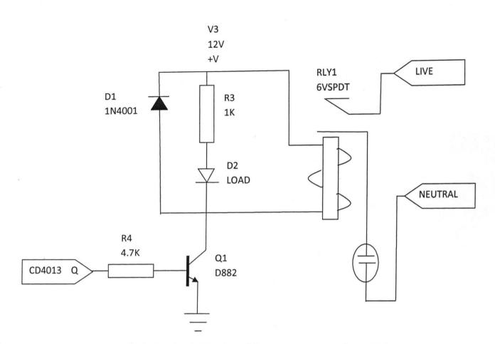
Fig.3.12: circuit diagram of the power control relay switch
