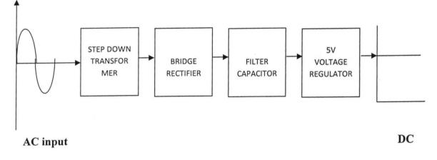
output Fig. 3.5 Block diagram of a power supply
