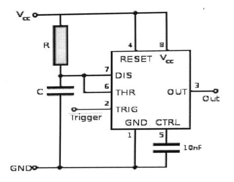
Fig. 3.10: circuit diagram of 555 monostable
