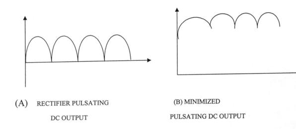
Fig. 3.7 filtering action of the capacitor
