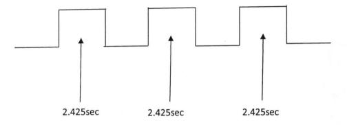
Fig 3.11 wave of the duration of clock pulse driving the T-flip-flop
