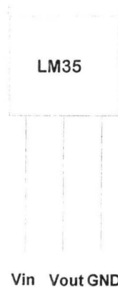
Fig. 2.2 Pin configuration of the LM35 [8]
