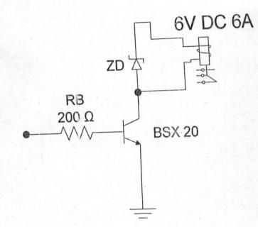
Fig 2.16 Driver Circuit
