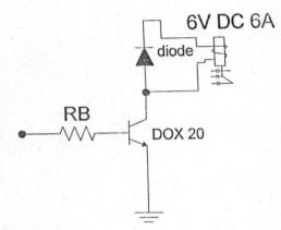
Fig. 2.8d Driver Circuit
