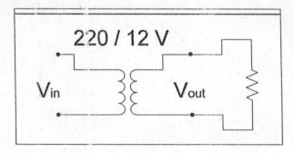
Fig.2.2 Transformation Circuit
