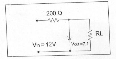
Fig. 2.6 Zener diode circuit
