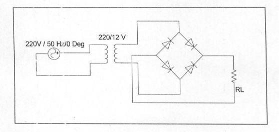
Fig. 29 Full Wave Bridge Rectifier Circuit
