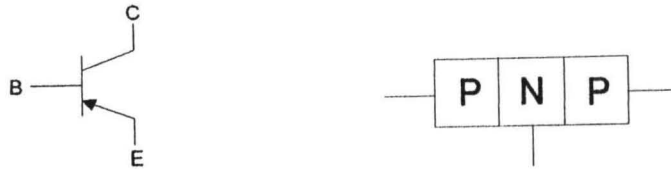
Fig 3.6a: Schematic symbol and circuit symbol of a PNP transistor
