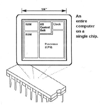
Fig. 3.9 Microcontroller Block diagram
