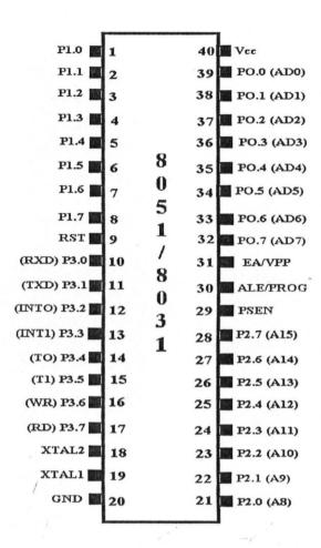
Fig.3.10 AT8952 Pin Function
