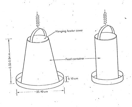
Figure 2: Tube feeders made of galvanised steel
