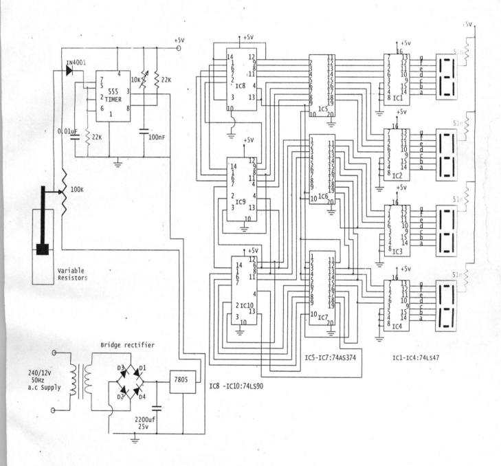
Circuit Diagram of a water leakage detector
