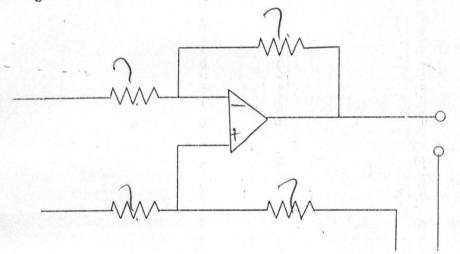
Voltage Difference Amplifier Circuit Diagram
