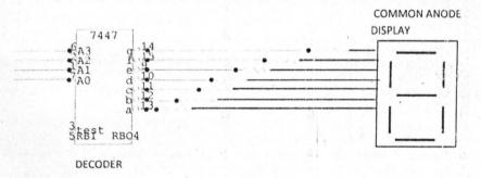
FIG 3.9 Circuit Diagram of BCD 7-Segment Decoder Driver with Common Anode Display
