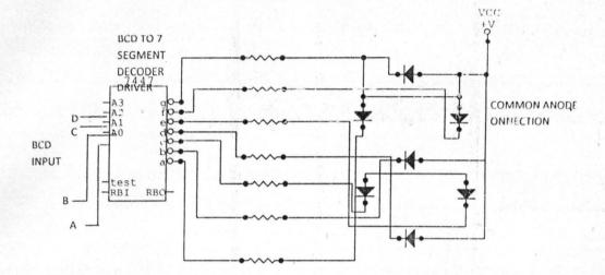
Fig 2:11 BCD to Seven Segment Divider Circuit Driver
