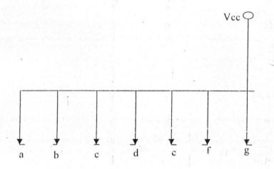
Common Anode Seven Segments Display Configuration.
