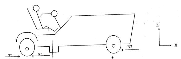
Considering the rear axle driven tractor above moving on a level ground, the forces acting on it from this view are:
