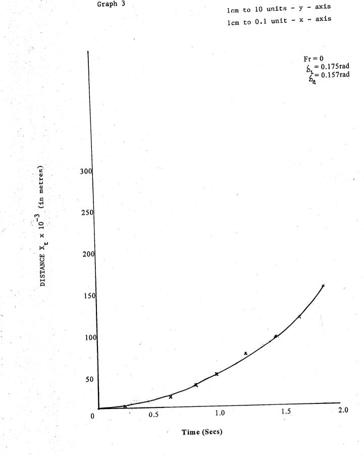
Fig 13: Effect of steering on tractor velocity
