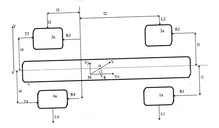
Figure 5: Top view of tractor with forces acting on it
