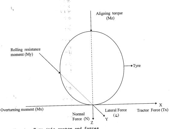
Figure 1. Tyre axis system and forces
