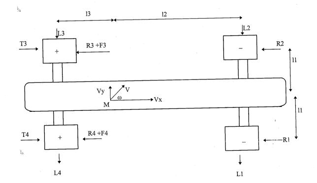
Figure 8 Braking forces and it's impact on tractor motion
