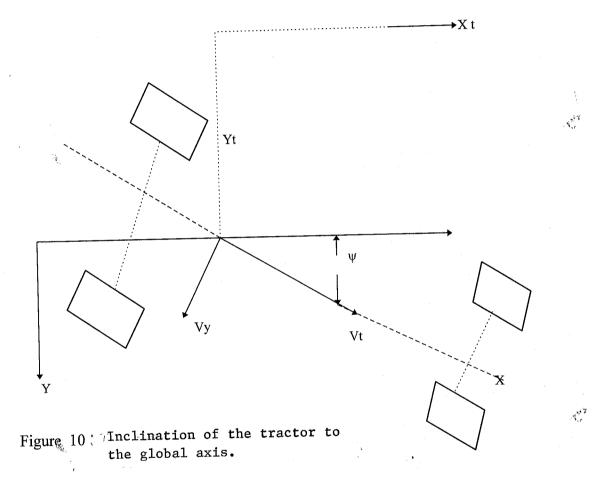
Assuming the tractors' x, y, system makes an angle  $\Psi$  with the global X, Y, Z system (see fig x), then the actual velocities in the global X, Y, Z directions will be:
