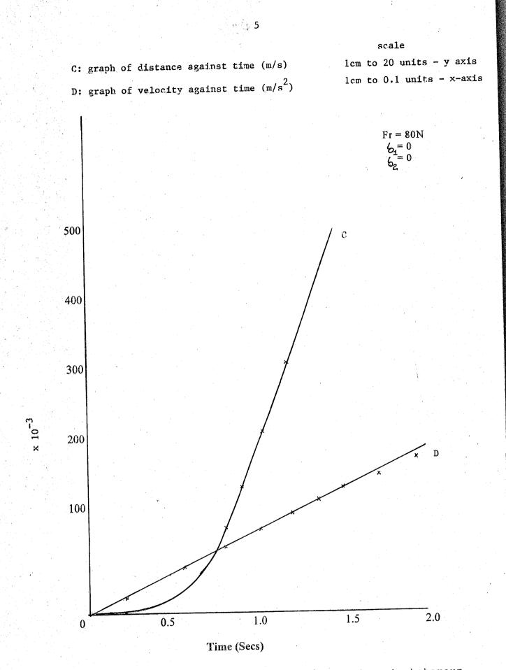
Fig 15: Low Breking force effect on the dynamic behavour of the tractor
