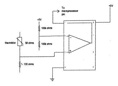
Fig 3.3 Circuit Diagram Of The Temperature Sensor
