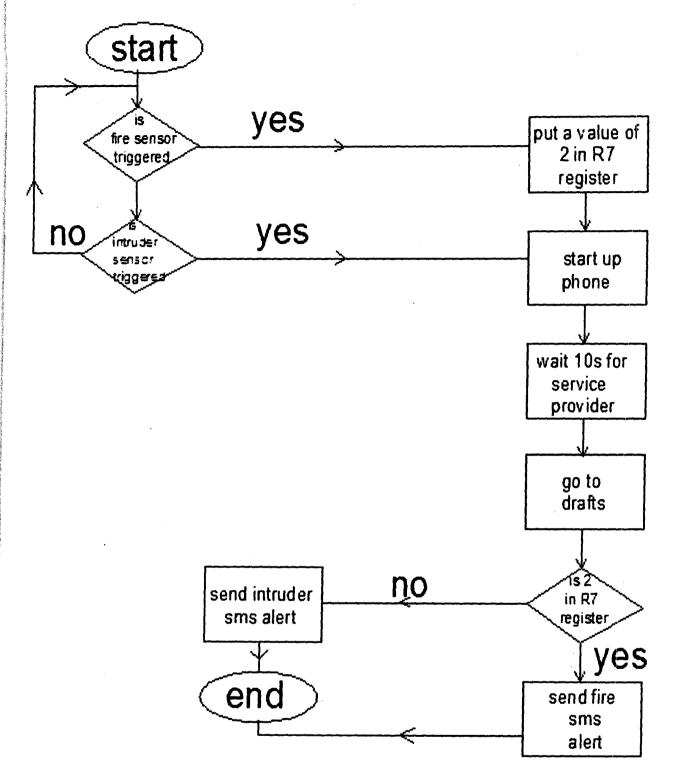
Fig 3.8 Microcontroller Flowchart
