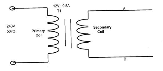
Fig 2.1 Step – Down Transformer
