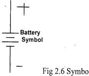
Fig 2.6 Symbolic diagram of battery
