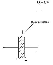
Fig 2.3 Symbolic Diagram of Capacitor
