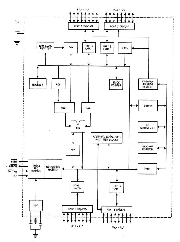
Fig 3.3 Internal Block diagram of AT89C51 Microcontroller
