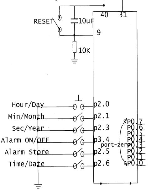
Fig 3.8 Interface of keypad with microcontroller
