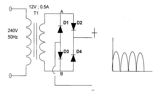
Fig 2.2 Bridge Rectifier Connected To Transformer And Its Waveform
