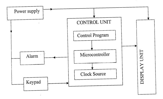
Fig 3.1 Block diagram of Microcontroller- based Digital clock and calendar
