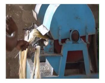
Plate I11: Banana Fiber Extracting Machine (Rahamaththulla et al., 2018).
