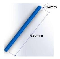
Figure F: Machine shaft
