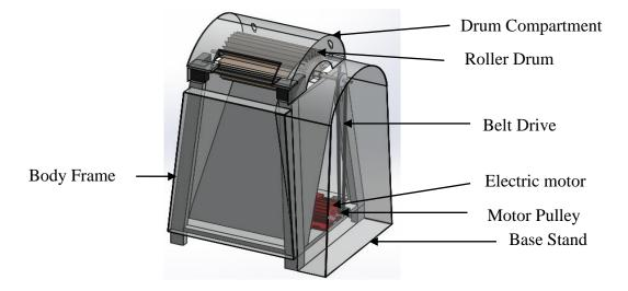
Figure 3.1: Proposed banana fiber machine to be fabricated
