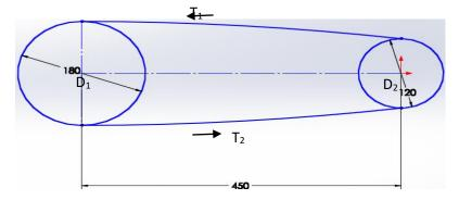
Figure 4.2: Belt Drive Mechanism on Shaft
