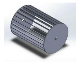
Figure E: Roller drum with beating blade
