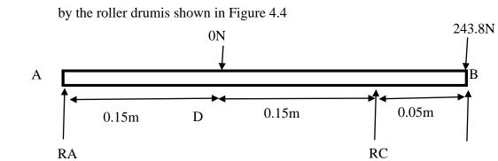
Figure 4.4: Shaft horizontal loading by roller drum
