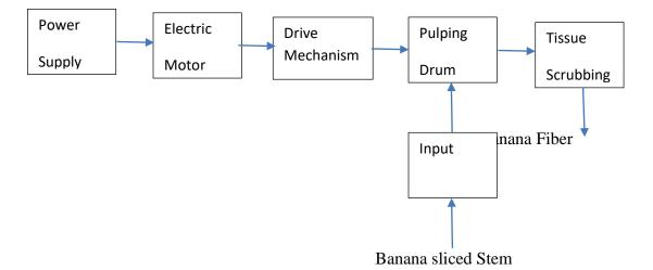
Figure 4.6: Block Diagram of Fiber Extractor Machine
