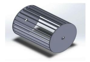
Figure 4.1; Rolling Drum with Beating Blade
