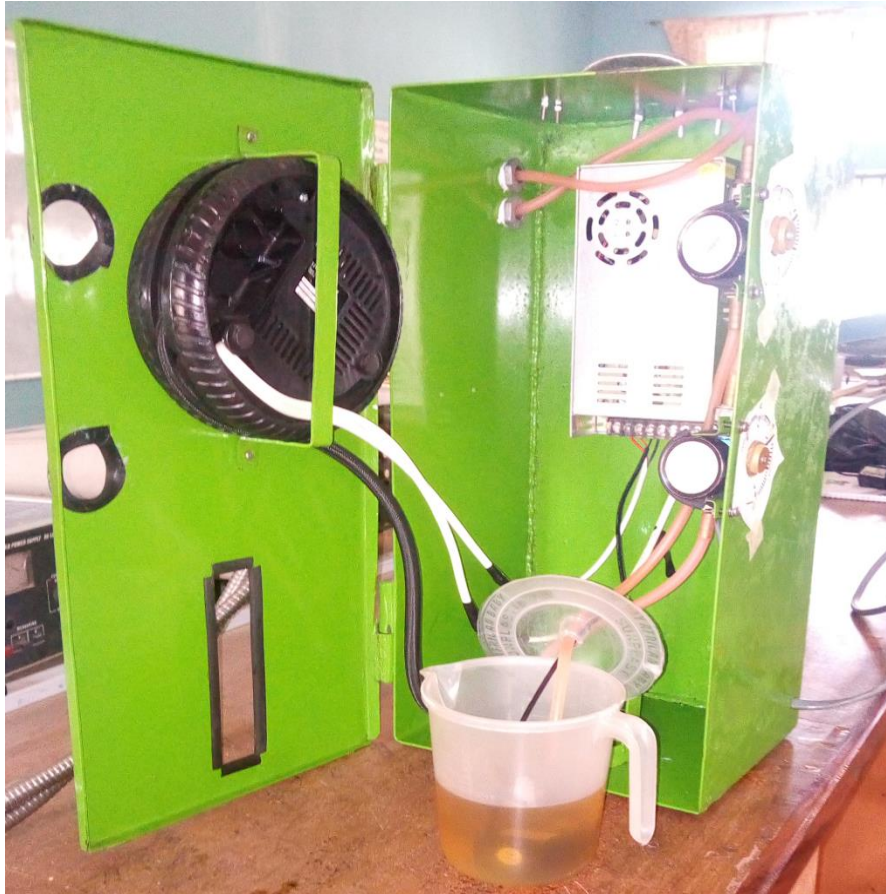
Plate II: Installation of pumping unit and the air compressor
