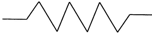
Fig 2.2 circuit symbol of a resistor
