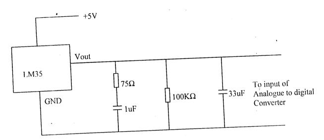
Fig 3.4 LM 35 Circuit connection
