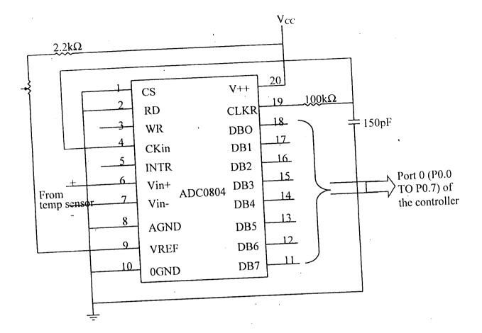
Fig 3.6; the interface between ADC and controller.
