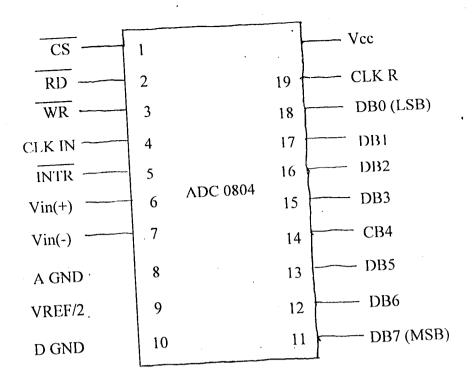
Fig 3.5 ADC 0804 pin out
