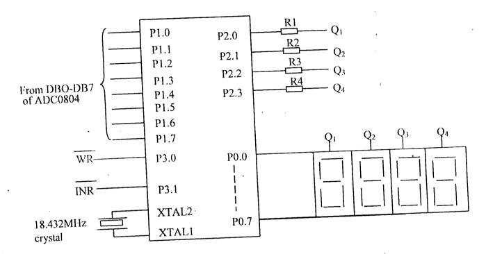
Fig 3.8 interface of microcontroller with other component
