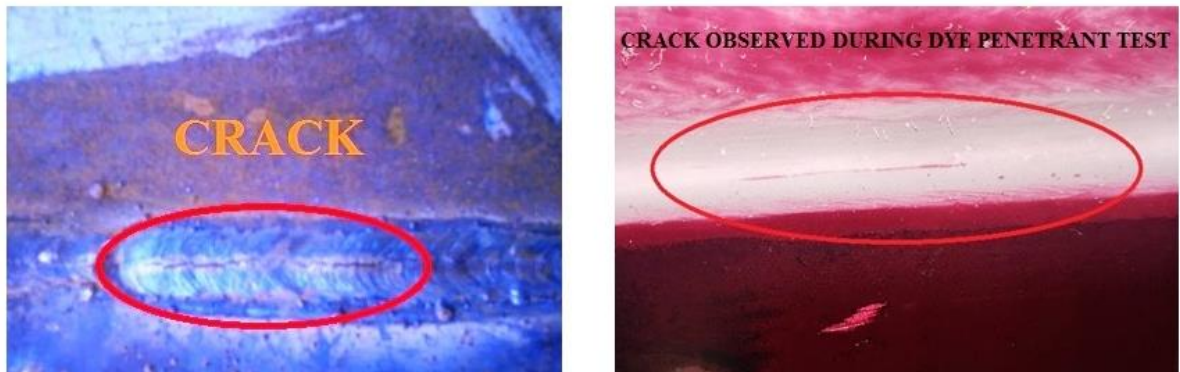
Figure 2.4: Cracks observed during dye penetration test. Source: (Anand, 2017)
