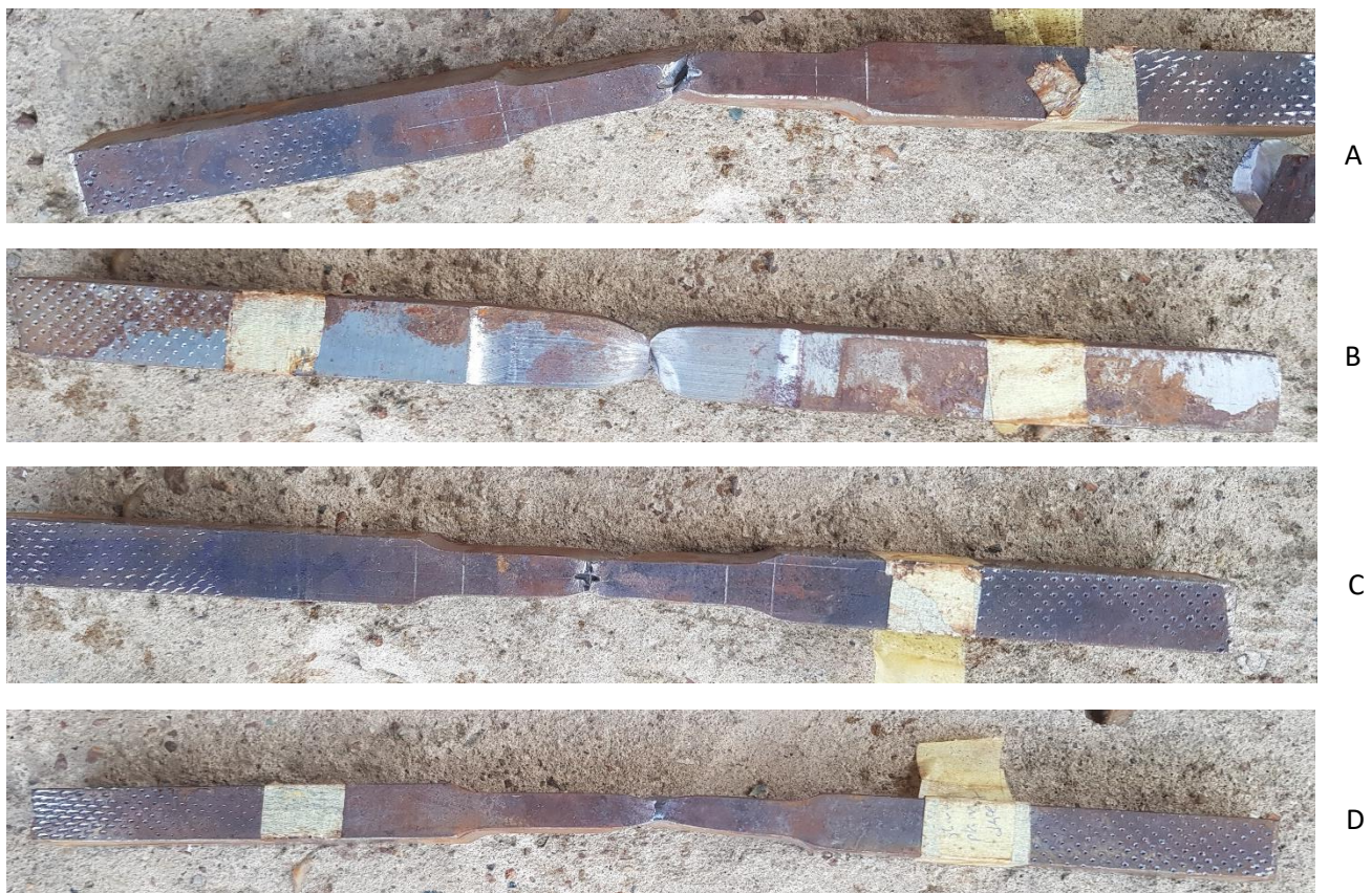
Figure 4.1: Weld and Parent Specimen subjected to destructive test (Tensile Test)
