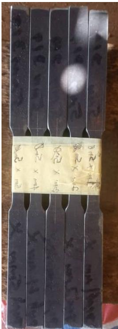
Plate IVa. Prepared Plain Tensile Samples with Artificial Defects
