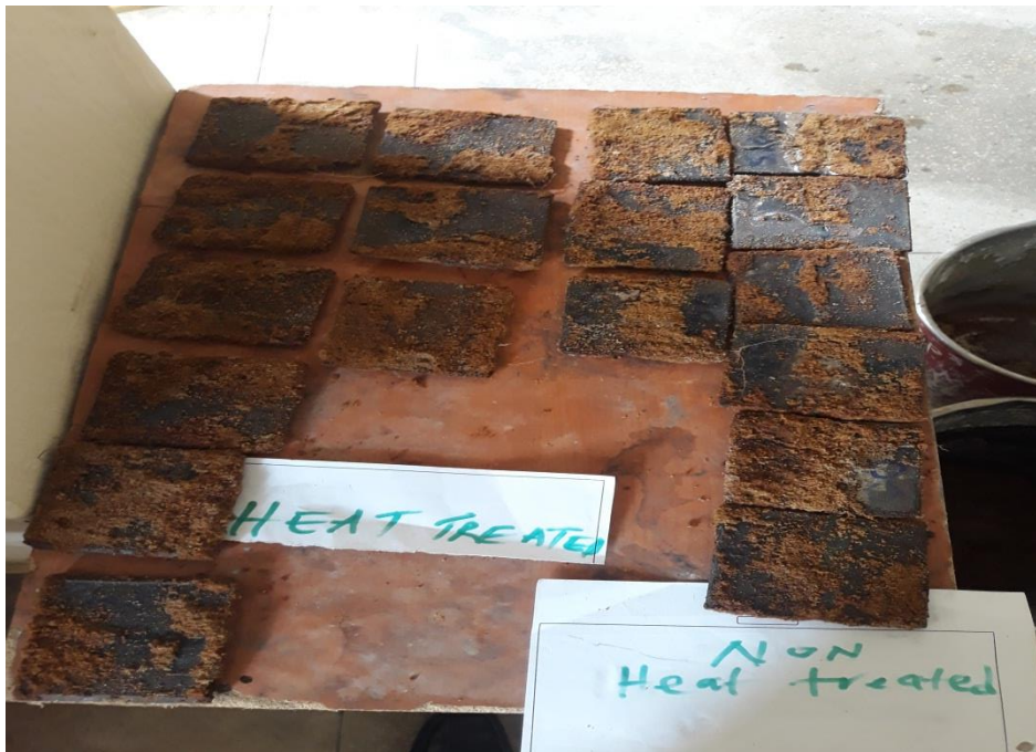
Plate XVIII: Typical corroded Samples
