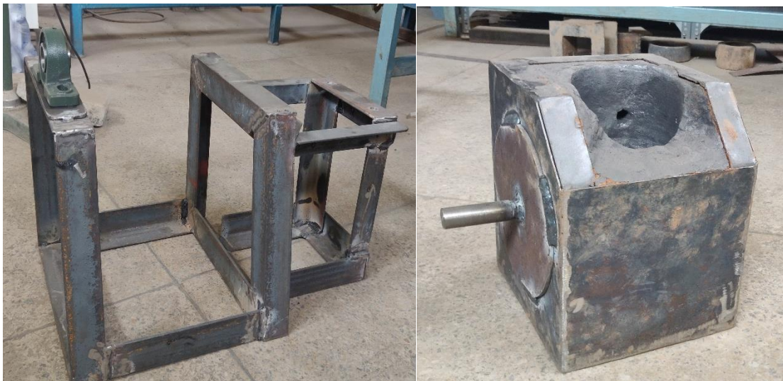
PLATE I: Frame and Crucible Housing for Induction Furnace
