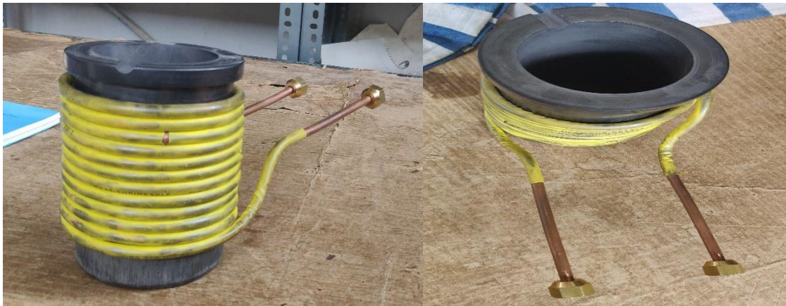
PLATE III: Heating Coil for Induction Furnace and Crucible
