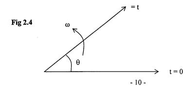
The instantaneous amplitude of the FM signal will be given by a formula of the form:  $V = A \sin[f(w_c, w_m)] = A \sin \phi - - - - (4)$ Where  $F(w_c, w_m)$  is some function of the carrier and modulating signal frequencies. This function represents an angle and will be called  $\theta$  for convenience.
