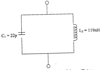
Fig 3.4: Tank circuit of the oscillator
