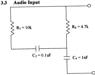
Fig 3.2: Circuit diagram of audio coupling network
