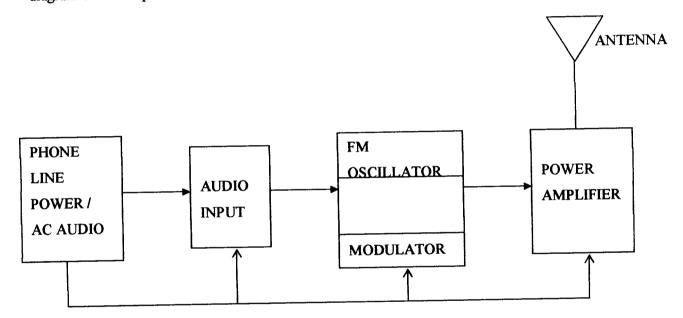
Fig 3.1: Block diagram of Telephone bug FM Transmitter
