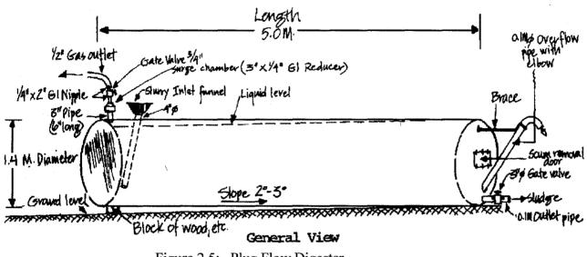
Figure 2.5: Plug Flow Digester
