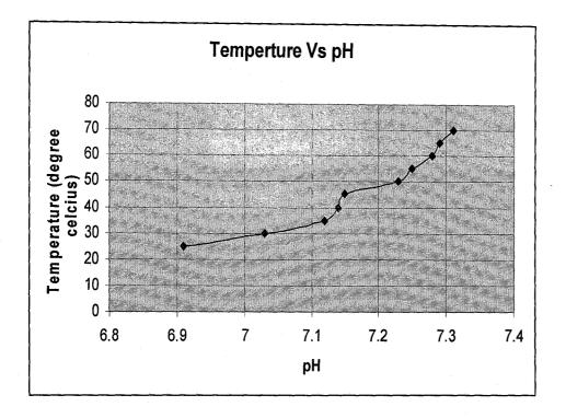
Figure 4.1: Temperature against pH on Biogas Production
