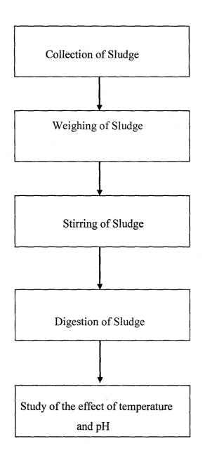
Figure 3.2: Flow Diagram of Biogas Production from Sludge.
