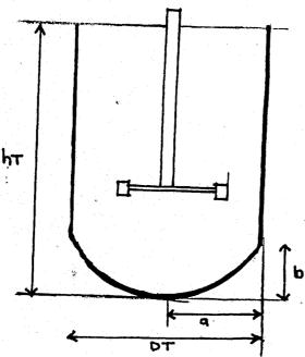
The diagram above is that of a reactor, where DT = Diameter of the reactor
