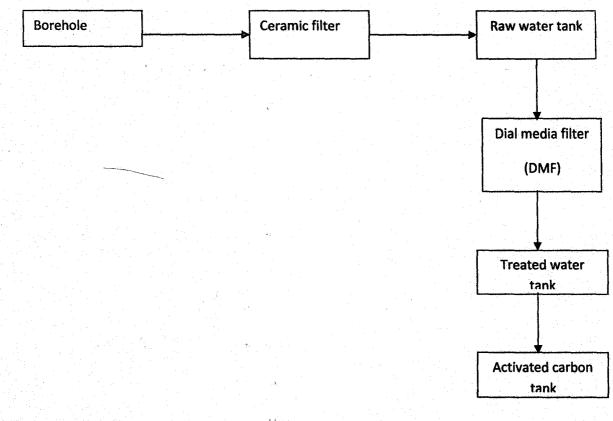
Fig 2.5 Flow chart of water treatment plant in brewery industry.
