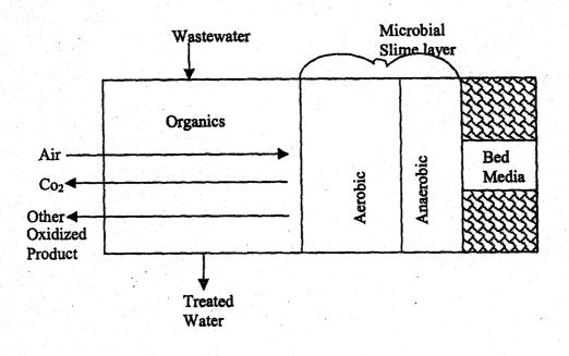
Fig 2.2 A schematic cross-section of the contact face of the bed median in a trickling filter. The treatment of sewage or other wastewater with trickling filter is the most well characterized treatment technologies.
