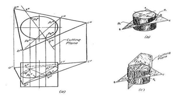
Figure 2.29 To find the intersection of a cylinder and a plane
