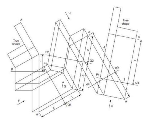
Figure 3.8 Projection of the true shape of a lamina
