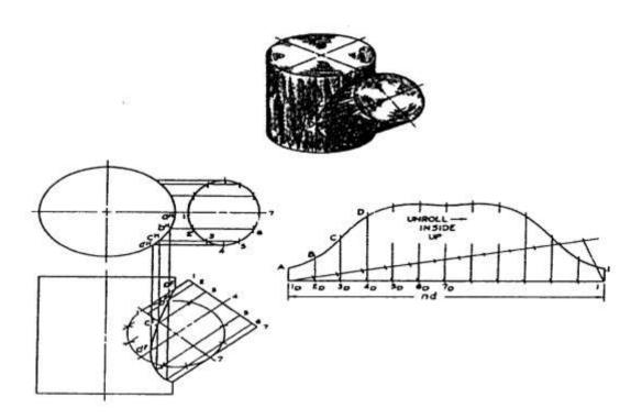
Figure 2.37 Intersecting cylinders
