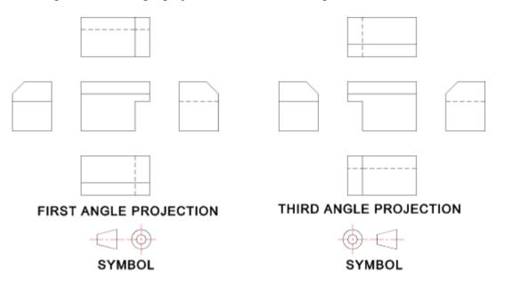
The symbol identifying the type of projection used should be placed in a space provided in the drawing block
