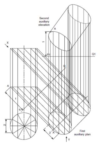
Figure 7 Auxiliary projections from a cylinder
