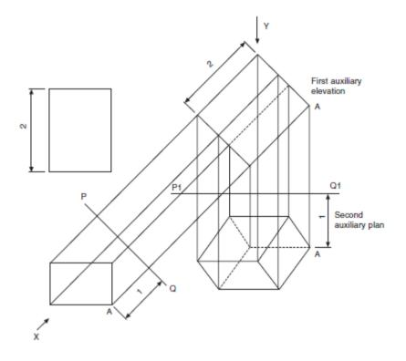
Figure 3.5 Isometric projection of a rectangular box from end view
