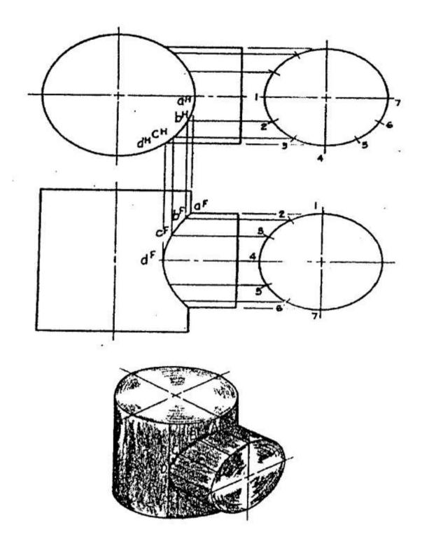
Figure 2.36 Intersecting cylinders
