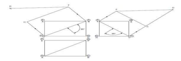
Figure 3.3 Projection of line from the front or end elevations
