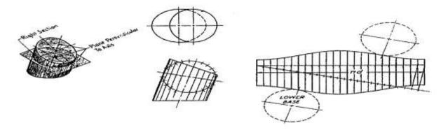
Figure 2.9 Development of an oblique cylinder
