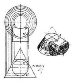
Figure 2.40 To find the intersection of Figure a cone and a cylinder Self-Assessment Exercise
