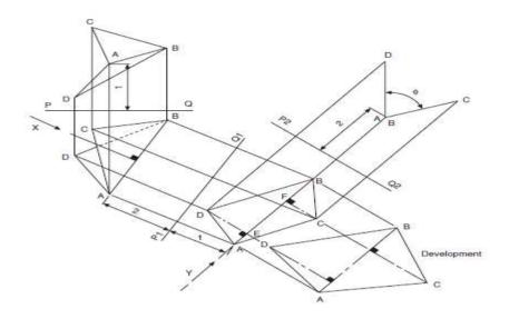
Figure 3.9 Projection of a lamina from a polygon
