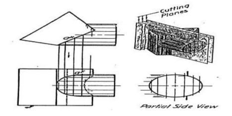
Figure 1.43 To find the intersection of a prism and a cylinder
