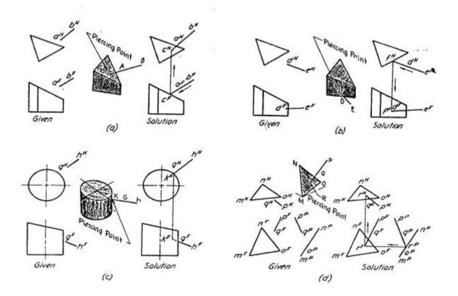
Figure 2.24 Determination of a piercing point by inspection
