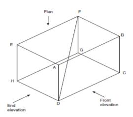
Figure 3.1 Line joining opposite corners of a box in space
