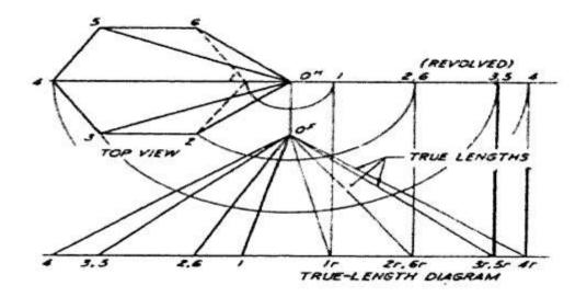
Figure 2.10. True-length diagram (the revolution method)
