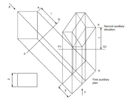
Figure 3.4 Isometric projection of a rectangular box from plan view
