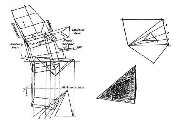
Figure 2.35 To construct a development using auxiliary view
