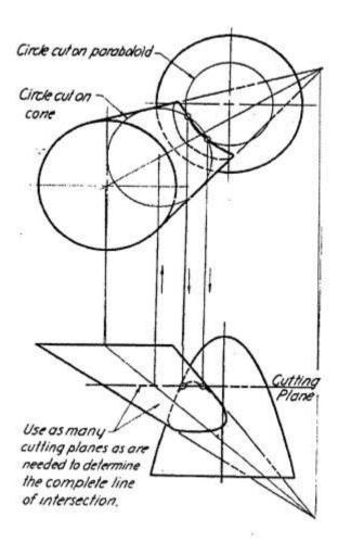
Figure 1.42 Intersecting cone and paraboloid
