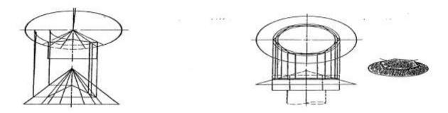
Figure 1.44 Intersecting cone and prism. Figure 145 Intersecting cone and hexagonal prism
