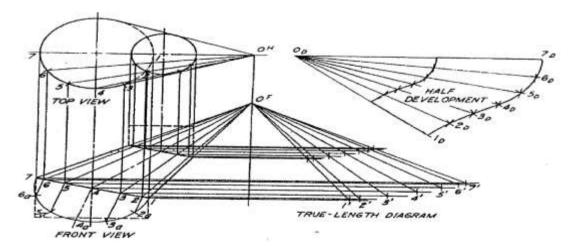
Figure 2.20 Transition piece connecting two pipes
