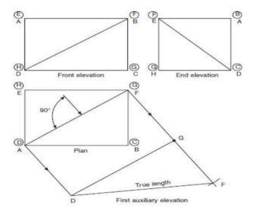
Figure 3.2 Projection of true length of line
