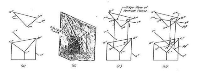
Figure 2.25 Use of a line-projecting plane
