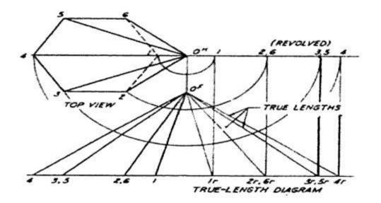
Figure 2.11 Development of a rectangular right pyramid
