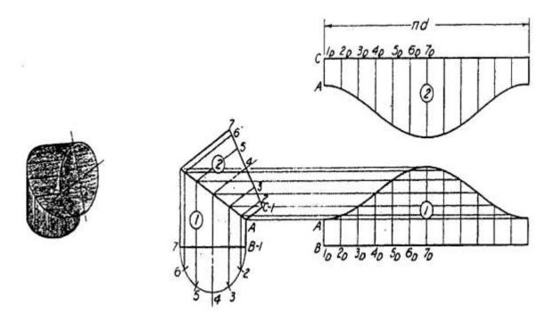
Figure 2.8 Two-piece elbow
