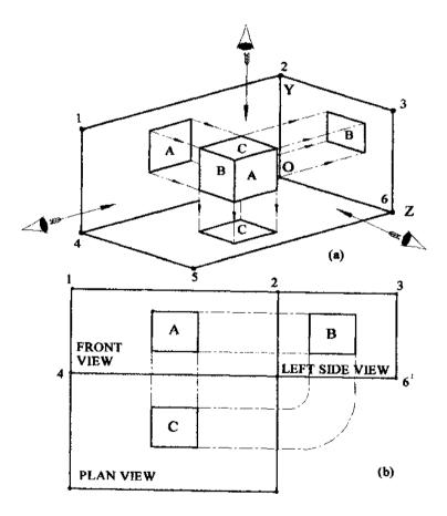
Fig. 89 The planes of projection in "First Angle".
