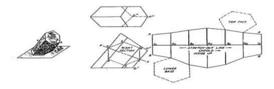
Figure 2.6 Development of an oblique prism
