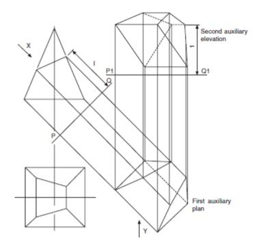
Figure 3.6 Projection of a truncated square pyramid
