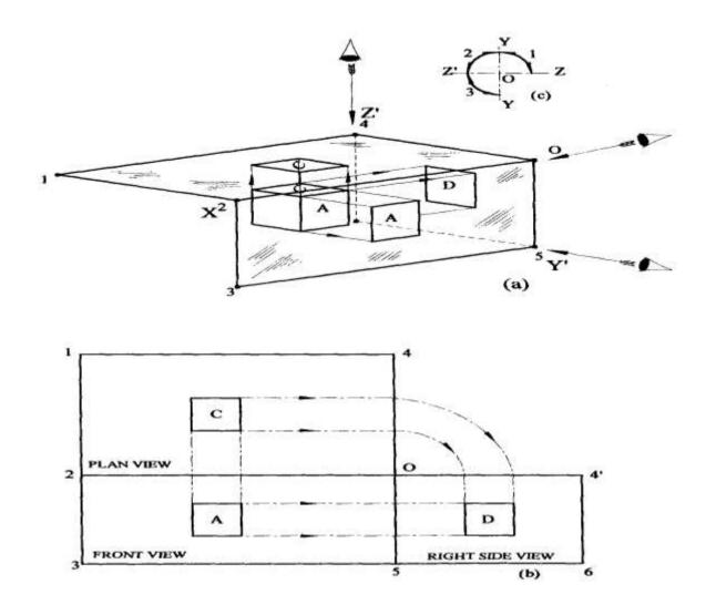
Fig. 90 The planes of projection in 'Third An
