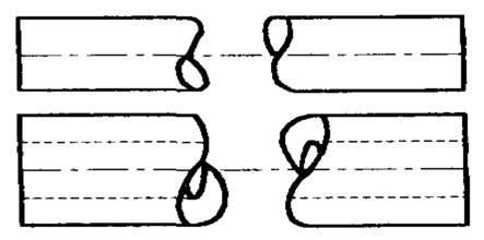
Fig. c Break lines for circular parts, solid or hollow
