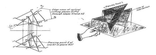
Figure 2.28 To find the intersection line of two planes
