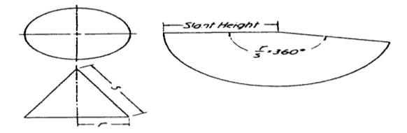
Figure 2.13 Development of a right cone
