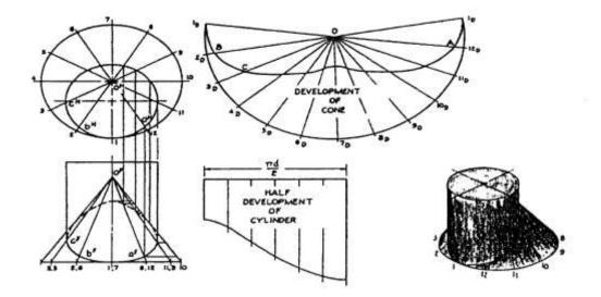
Figure 1.39 Intersecting cylinder and cone
