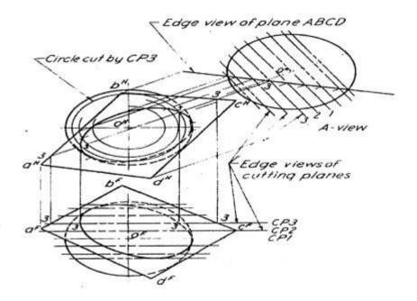
Figure 2.31 To fined the intersection of a sphere and an oblique plane
