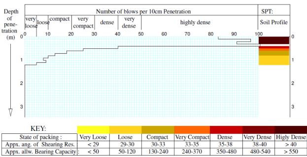
Fig. 5. DCPT Result for test location one (CH 18+600).
