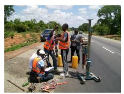
Fig. 4. Dynamic Cone Penetration test.
