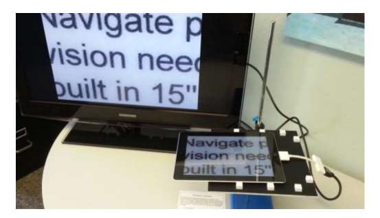
Figure 2.3 Magnification system
