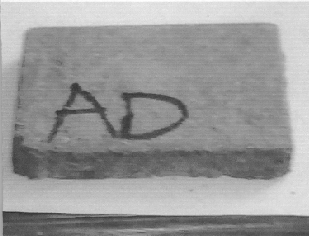
Plate 4.4 Particle Board made from a mixture of Sawdust and Sugarcane Bagasse
