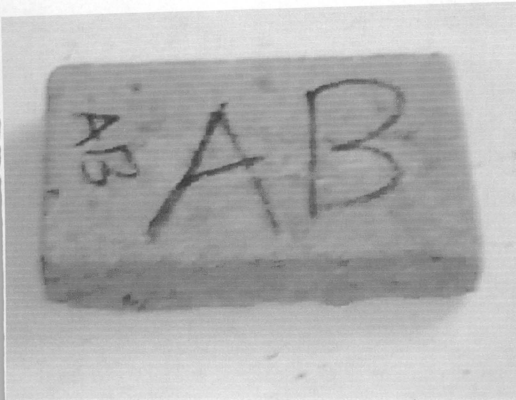
Plate 4.4 Particle Board made from a mixture of Sawdust and Sugarcane Bagasse
