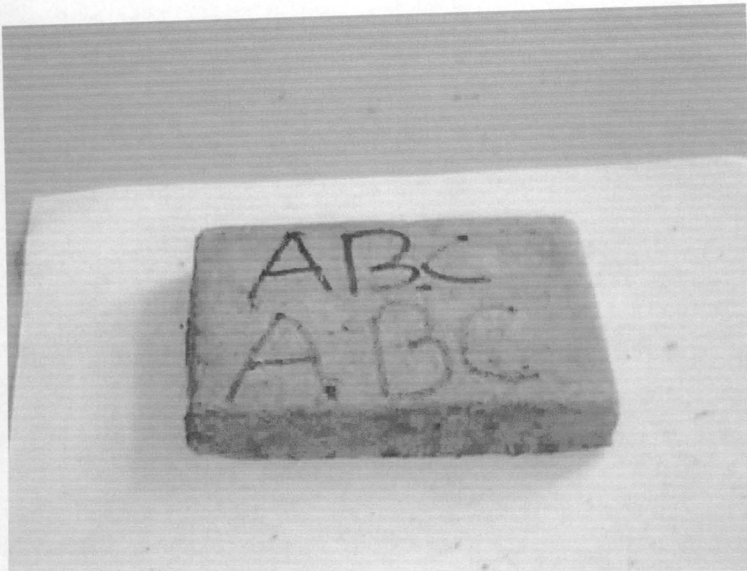
Plate 4.7 Particle boards made from a mixture of Sawdust, Sugarcane bagasse and Melon shell
