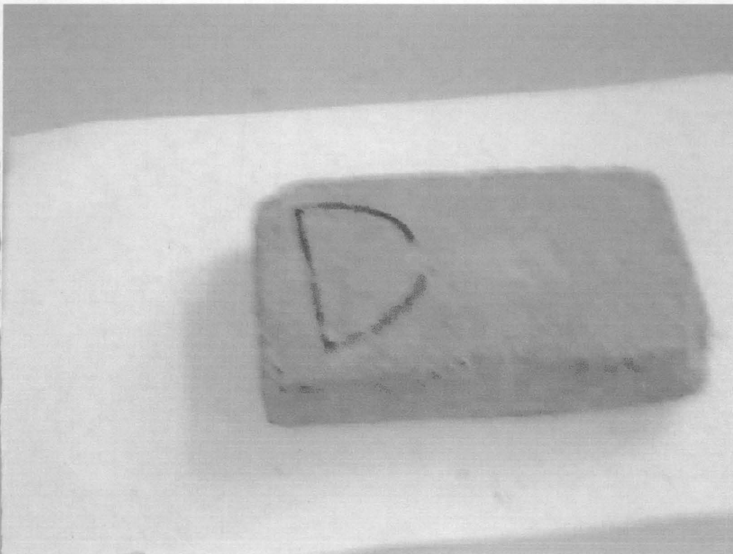
Plate 4.2 Particle Board made from Sugarcane Bagasse
