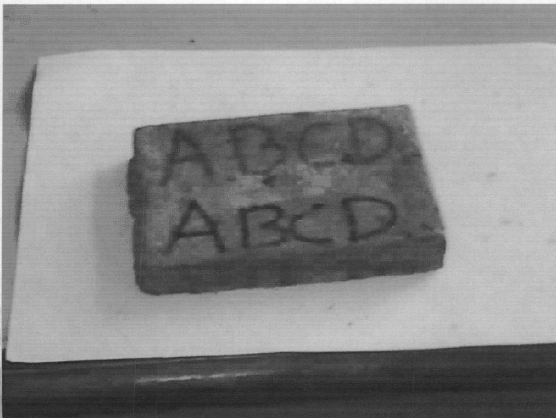
Plate 4.8 Particle board made from a mixture of Sawdust, Sugarcane bagasse Melon shell and Rice Husk
