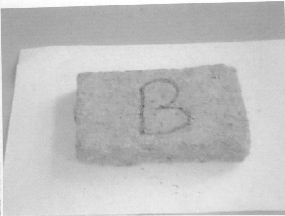
Plate 4.2 Particle Board made from Sugarcane Bagasse
