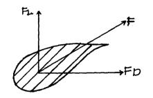
FIG. 3.2 Forces Acting on a particle Under dir Current.
