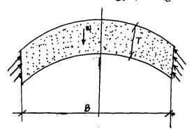
FIG : 3.7 FREE - BODY DIAGRAM OF A MASS OF GRANULAR MATERIAL FORMING AN
