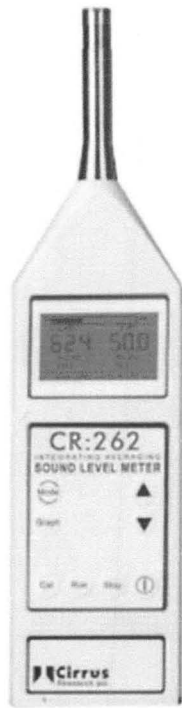
Fig. 3.2 An integrating-averaging sound level meter complying with IEC 61672:2003
