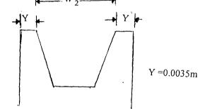
Figure 4.8 Cross-section of pulley
