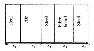
Fig. 4.23 Furnace Casing Wall thickness
