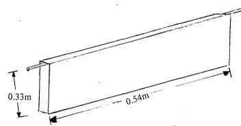
Fig.4.39 Material discharge door.
