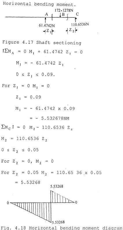
The maximum bending moment at point B is 4,852239 That at c is given by
