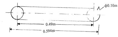
Fig.4.27 Conveyor Sprockets and Chains
