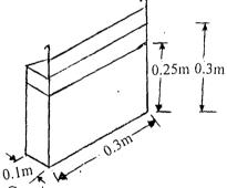
Fig: 4.21 Combustion Grate
