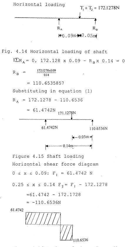
Figure 4.16 Horizontal shear Force diagram
