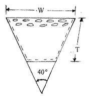
Figure: 4.3 standard selection V-belts. For V-belt A, the following are the data of its sections. Usual load of drive 0.75 - 5 kw. Recommended minimum pitch diameter d = 75 mm Nominal top width w = 13mm Nominal thickness T = 8mm Weight per meter = 0.106 kg/m
