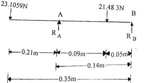
Fig. 4.9 vertical loading of shaft  $\Sigma vf = R_A + R_B - (23.1059 + 21.483) = 0$
