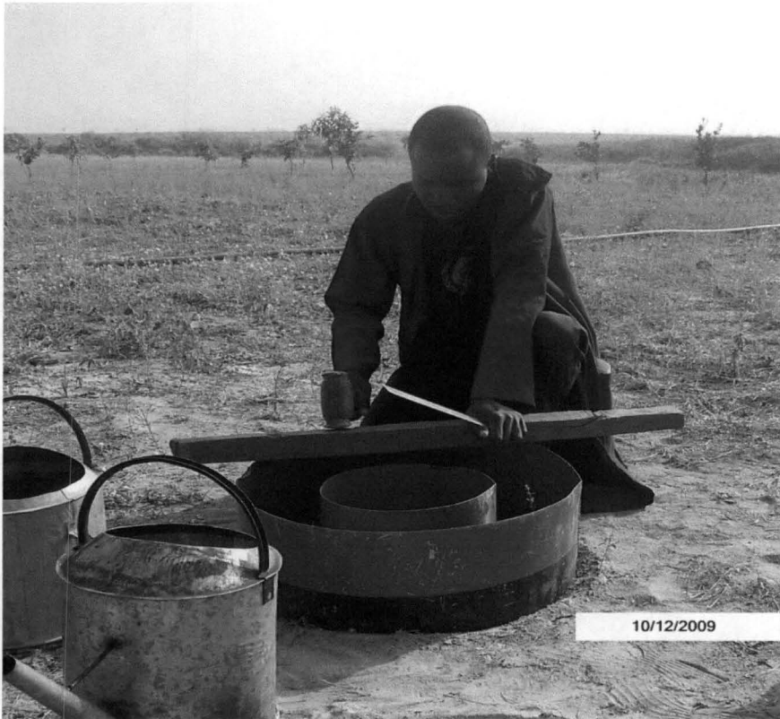
Plate 3.1 Installation of the Infiltrometer
